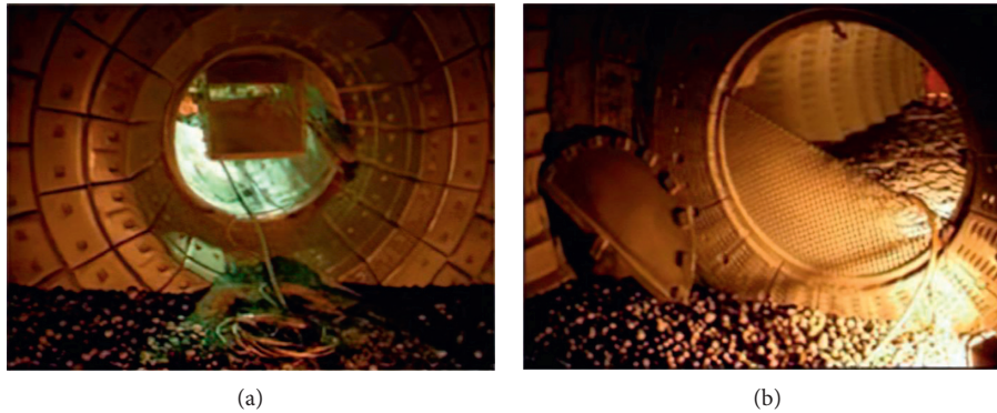
FIGURE 5: Two-compartment tube ball mill. (a) Compartment 01. (b) Compartment 01/02 and separating diaphragm [26].
