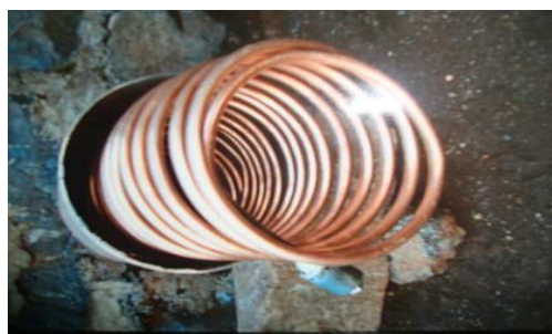
Figure 3: Heat exchanger during assembly
