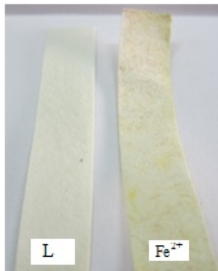
Figure 11: Test paper kit of receptor L in presence of \text{Fe}^{2+} ion.
